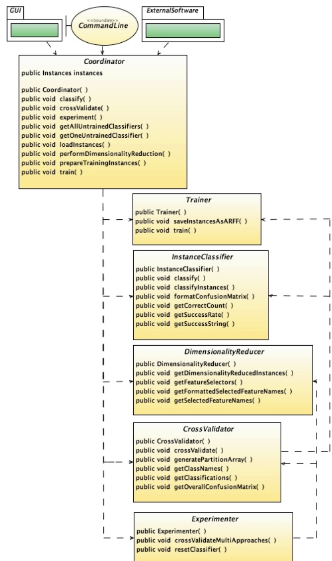
Figure 1. Structure of ACE's main processing classes. The Coordinator class provides an exclusive interface through which ACE's main functionality can be accessed. Arrows indicate interactions between classes. All public methods are listed, but parameters are omitted from method declarations to save space.
